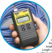
The Length Mode measures the length of a cable by measuring its capacitance and using the capacitance per length (length constant). Length can be measured with or without remote attached.
